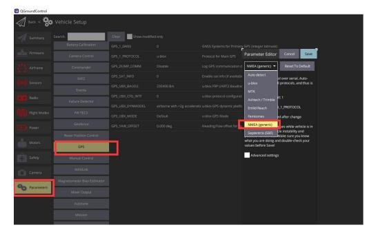
Please note that the above parameters assume you have connected the positioning and orientation module to the GPS MODULE interface. If you are using a different port, you must configure the baud rate and protocol using the respective parameters.
