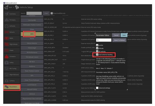
**GPS\_YAW\_OFFSET:** If the primary antenna is located at the front, set the yaw offset to 0. Angles increase in a clockwise direction. If the primary antenna is on the right side of the vehicle and the secondary antenna is on the left side, set the offset to 90 degrees.
