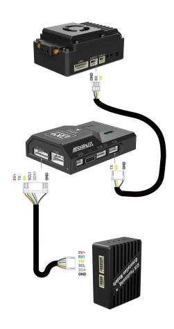
Refer to the diagram above to connect the RTK mobile module to the flight controller, while the flight controller is connected to the airborne data link.
