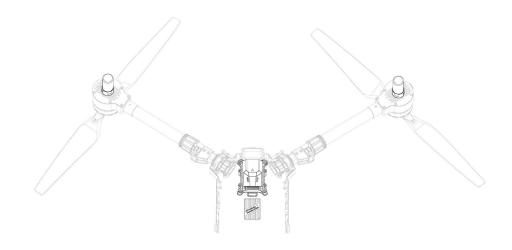
Refer to the image above to securely mount the RTK mobile end on the aircraft body, ensuring it does not wobble. The arrow on the RTK module should align with the installation direction of the
